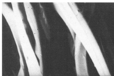
Figure 9 Scanning electron micrograph of treated polyester fabric with sodium propoxide solution. Conditions: 1M sodium propoxide, padding technique, pick up 100%, 25^{\circ}\text{C} , 24 h.
