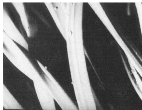
Figure 8 Scanning electron micrograph of treated polyester fabric with sodium ethoxide solution. Conditions: 1M sodium ethoxide, padding technique, pick up 100%, 25^{\circ}\text{C} , 24 h.
